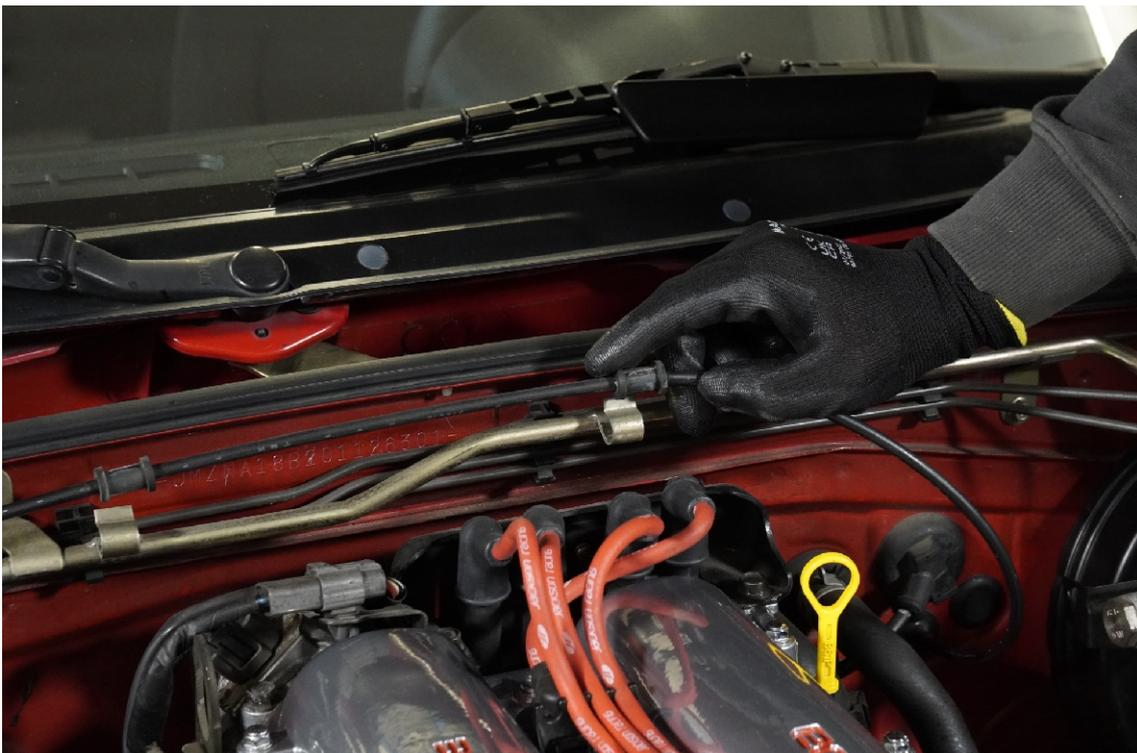
3. Disconnect the hose from the intake manifold:
