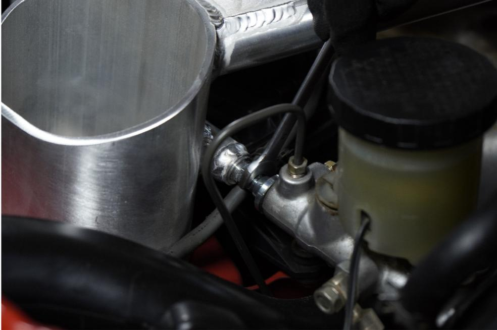
*The ball joint must be adjusted to stabilize the brake booster without exerting unnecessary pressure on the brake master cylinder.*
