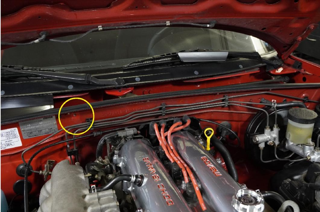
2. Attach the support plate with a screw in the existing thread. Tighten the screw only hand-tight so that the plate can still be aligned.
