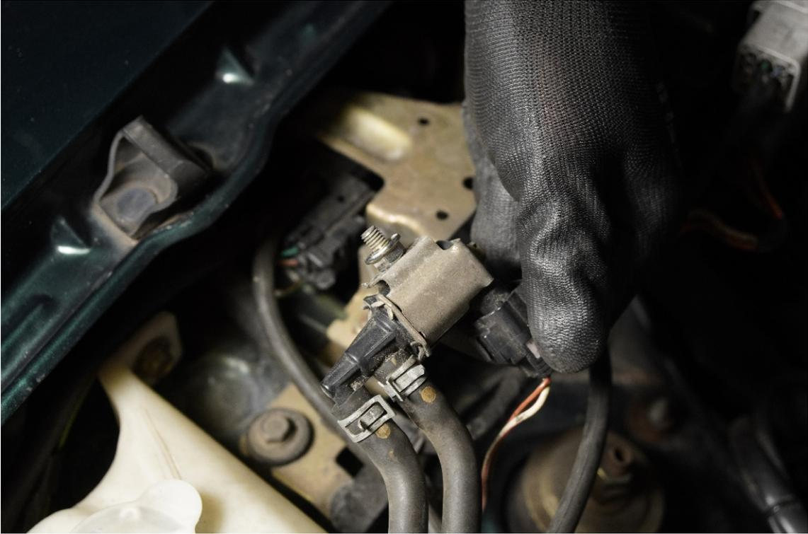
5. Removing the vacuum lines:
