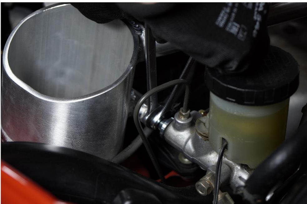
3. Check that the ball joint is correctly seated and the locknut is securely tightened.
